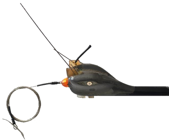
Figure 7 : Balise SPLASH10-F-321 (Fastloc®) (A. Rohr-APECS)
